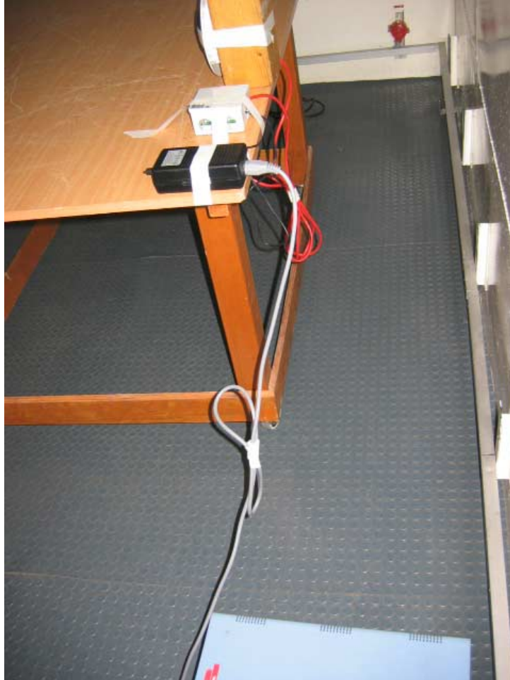
Photograph No.9 Setup for conducted emissions measurements, side view EUT operating at 433.9 MHz
