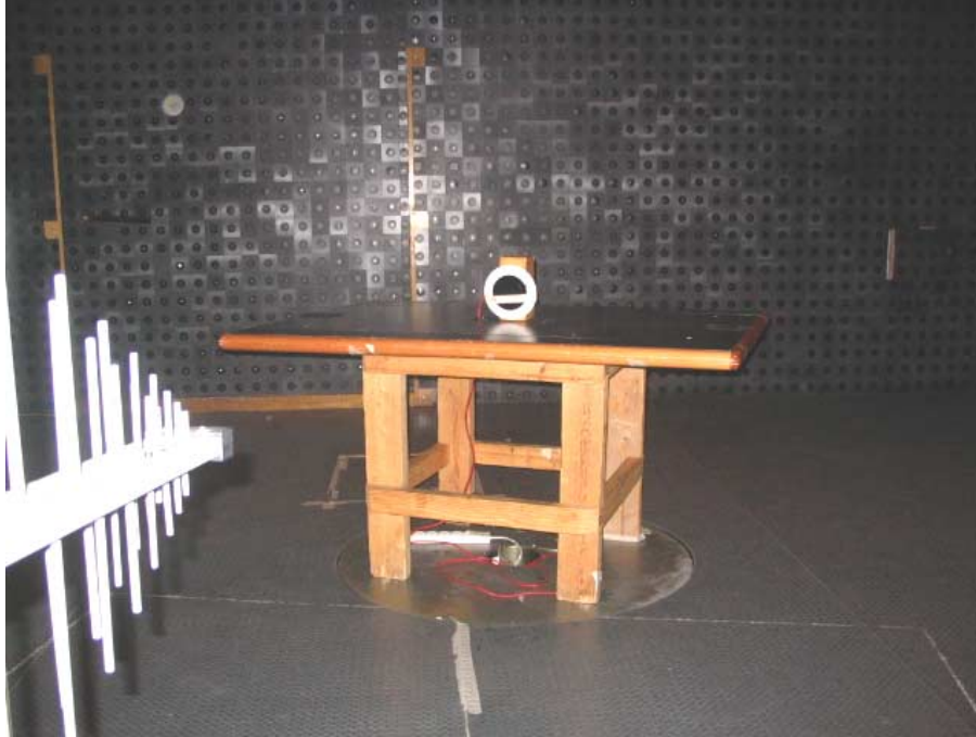
Photograph No.10 Setup for unintentional radiated emission measurements EUT operating at 433.9 MHz
