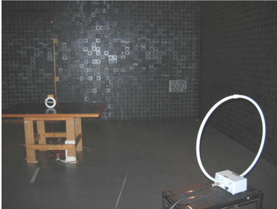
Photograph No.5 Setup for spurious emission field strength measurements below 30 MHz EUT operating at 433.9 MHz
