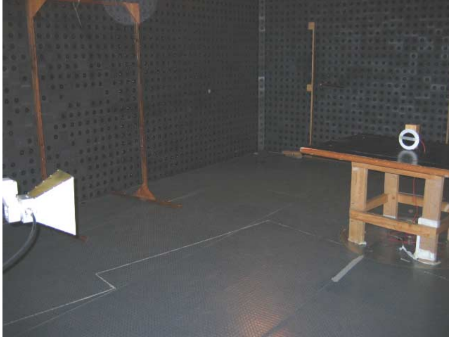
Photograph No.7 Setup for spurious emission field strength measurements above 1000 MHz EUT operating at 433.9 MHz
