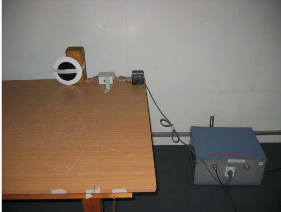
Photograph No.8 Setup for conducted emissions measurements, front view EUT operating at 433.9 MHz
