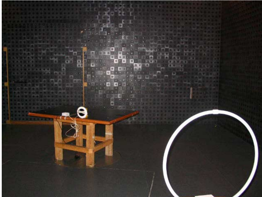
Photograph No.1 Setup for spurious emission field strength measurements in anechoic chamber below 30 MHz EUT operating at 125 kHz
