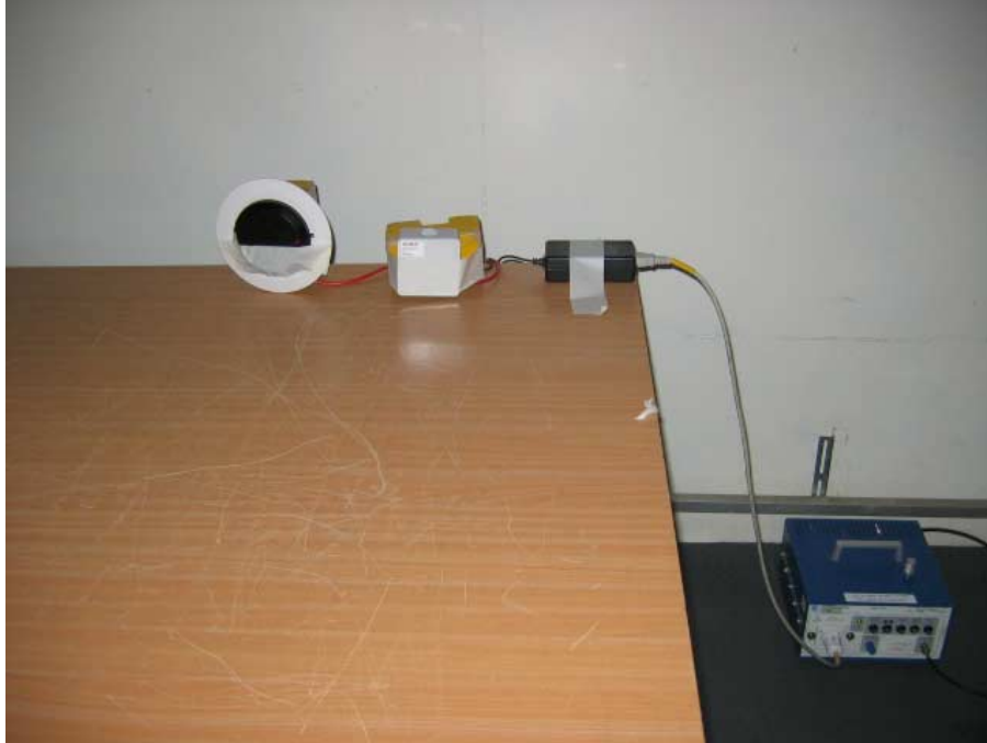
Photograph No.3 Setup for conducted emissions measurements EUT operating at 125 kHz
