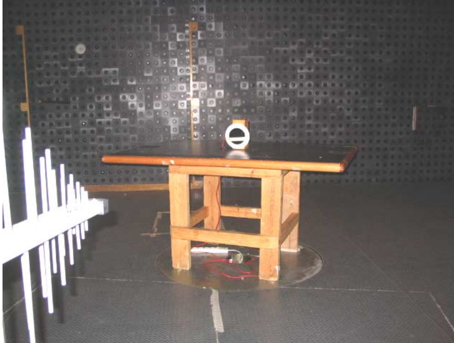
Photograph No.6 Setup for spurious emission field strength measurements from 30 MHz to 1000 MHz EUT operating at 433.9 MHz
