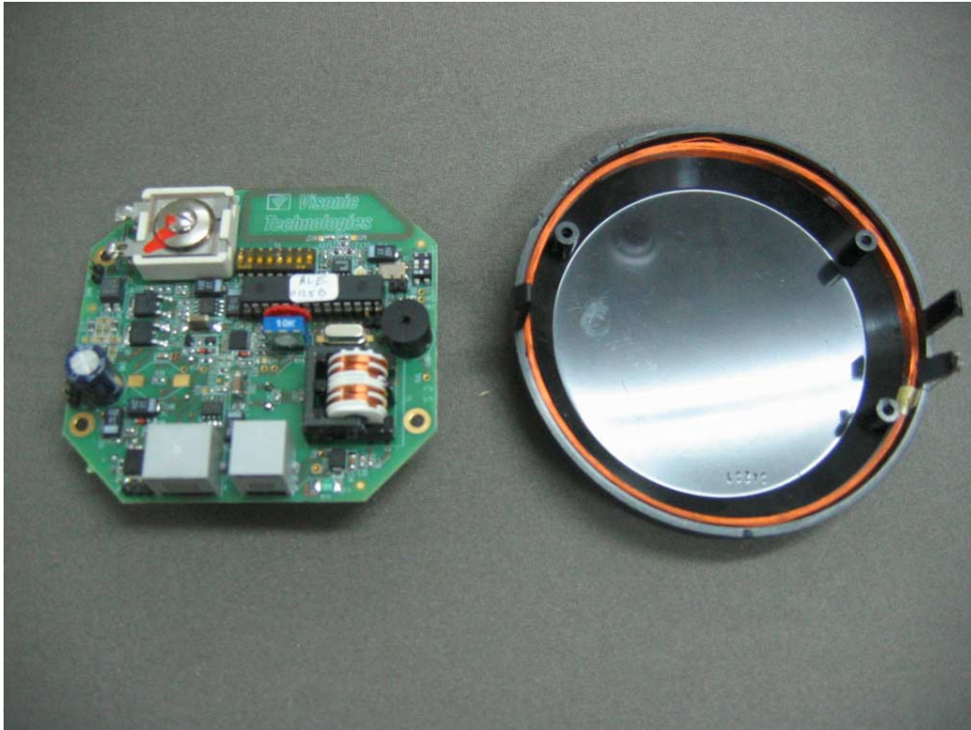
Photograph No.5 LF Exciter Antenna compartment removed from PCB
