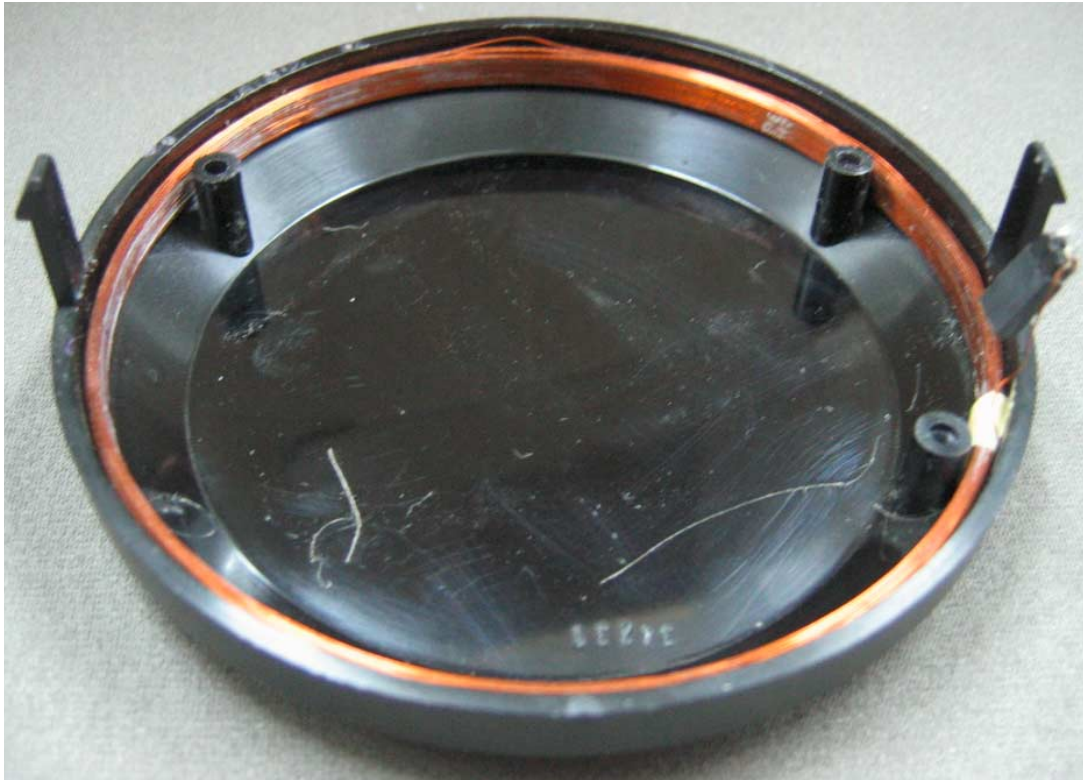
Photograph No.6 LF Exciter Antenna compartment
