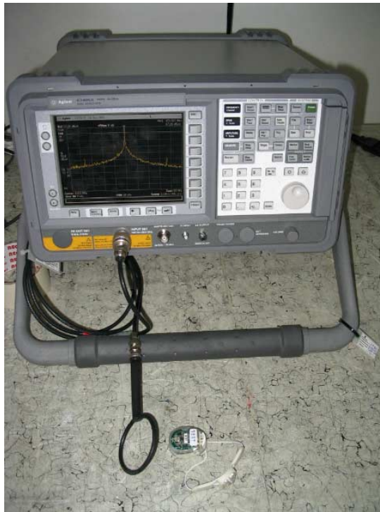
Photograph No.5 Setup for occupied bandwidth test
