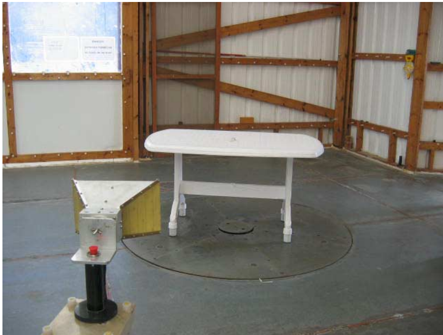
Photograph No.4 Setup for spurious emission field strength measurements at OATS
