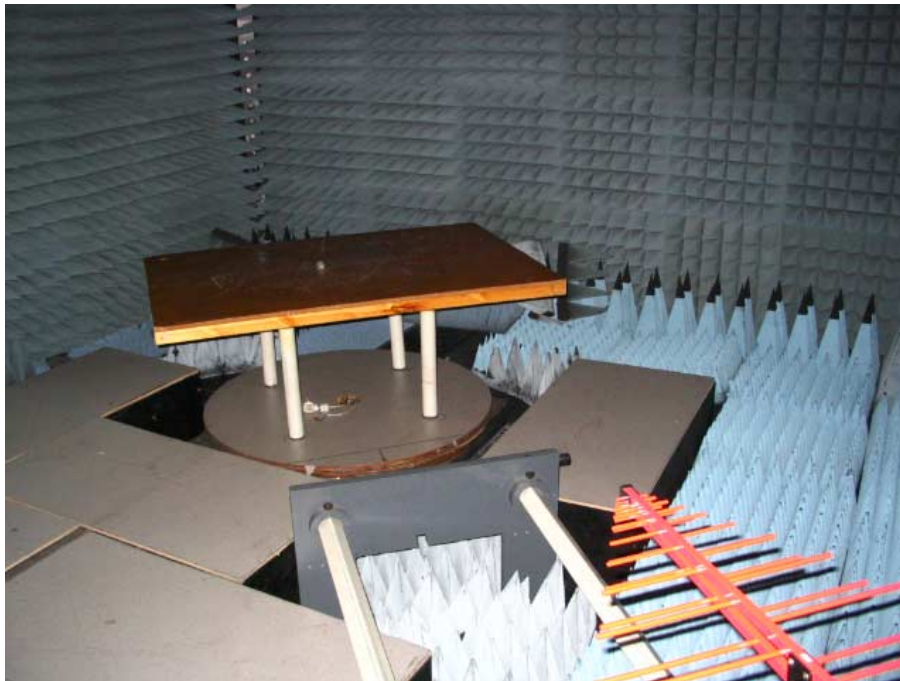
Photograph No.6 Setup for unintentional radiated emission measurements in anechoic chamber
