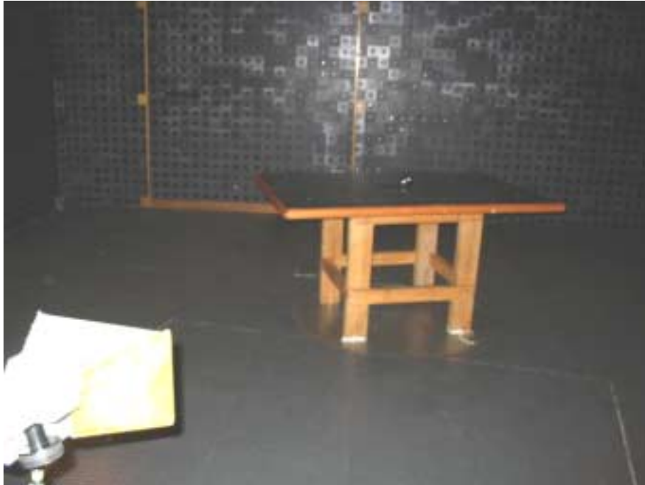
Photograph No.4 Setup for spurious emission field strength measurements in anechoic chamber above 1000 MHz
