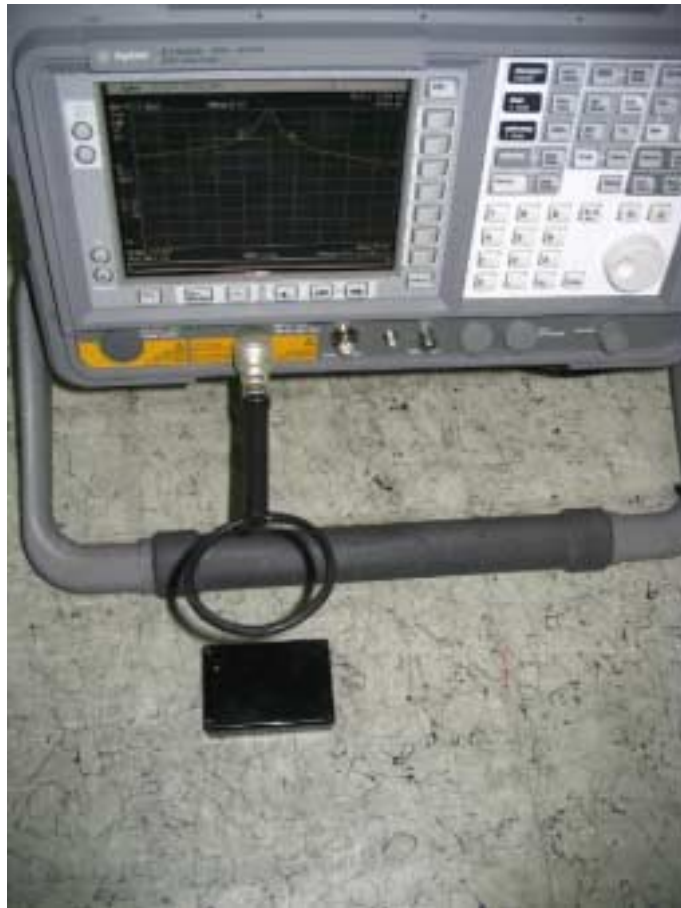
Photograph No.6 Setup for occupied bandwidth test
