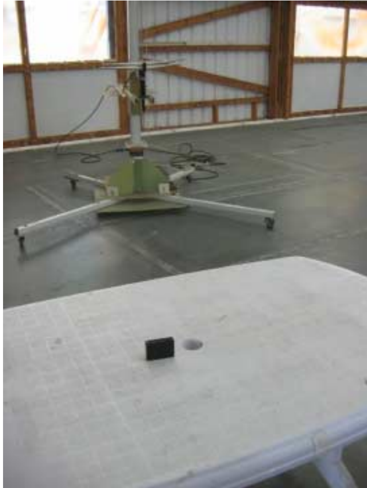
Photograph No.3 Setup for spurious emission field strength measurements at OATS from 200 to 1000 MHz
