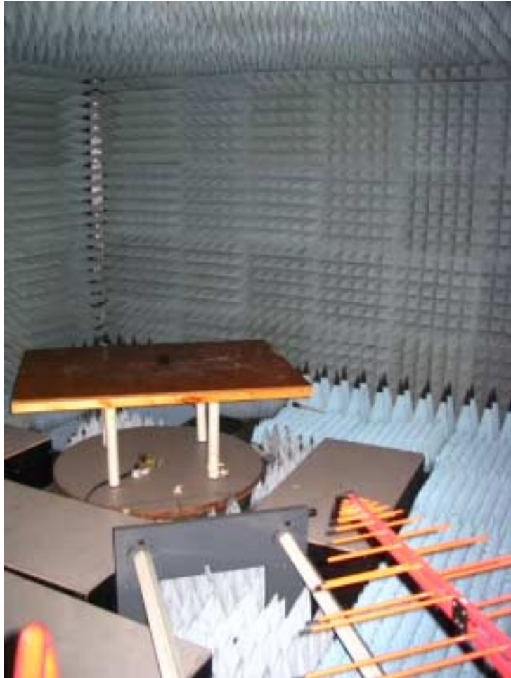
Photograph No.2 Setup for spurious emission field strength measurements in anechoic chamber from 30 to 1000 MHz
