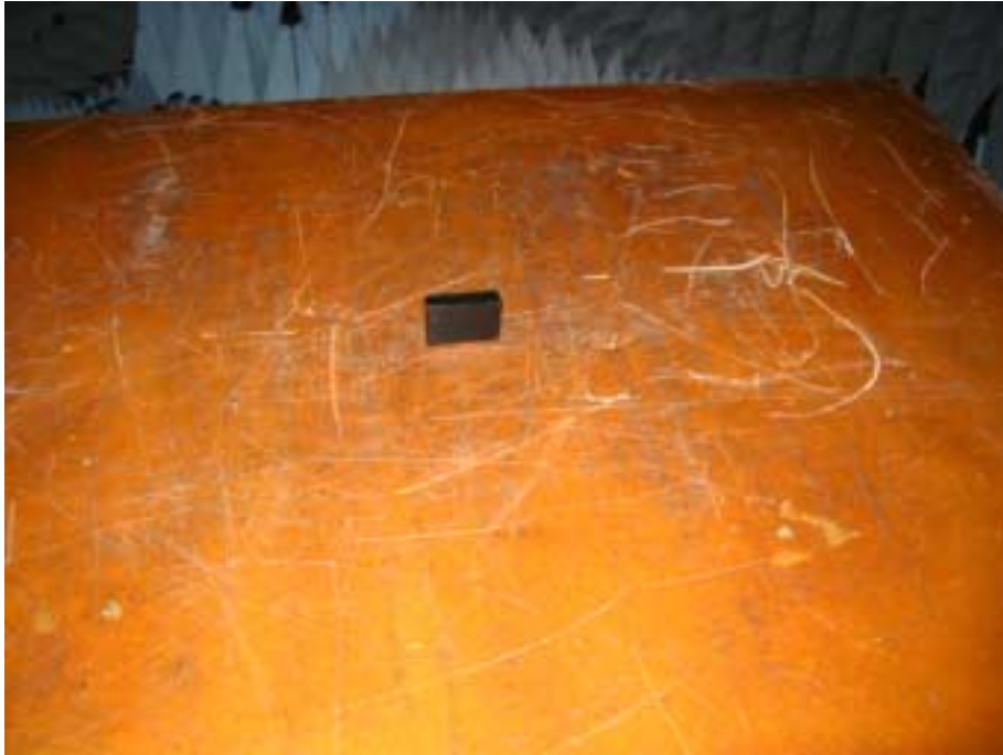
Photograph No.8 Setup for radiated emission measurements in anechoic chamber, EUT view
