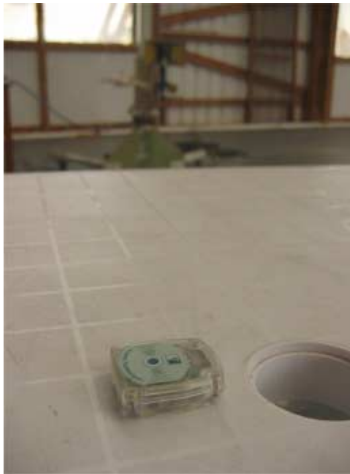
Photograph No.5 Setup for spurious emission field strength measurements at the OATS, close view
