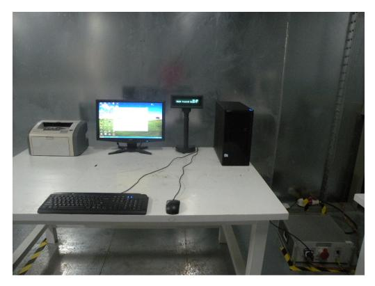
Radiated Emission Test Setup in Chamber
