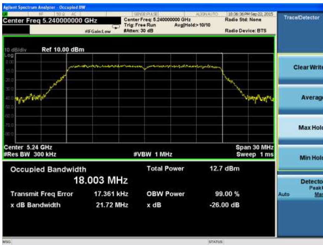
Test Plot For 802.11n(HT20)-26dB BW-5240M-Chain 0
