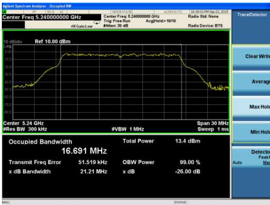
Test Plot For 802.11a-26dB BW-5240M-Chain 0
