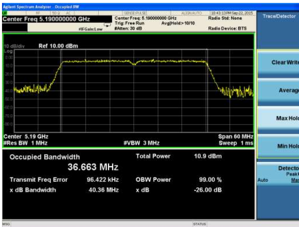
Test Plot For 802.11n(HT40)-26dB BW-5190M-Chain 0
