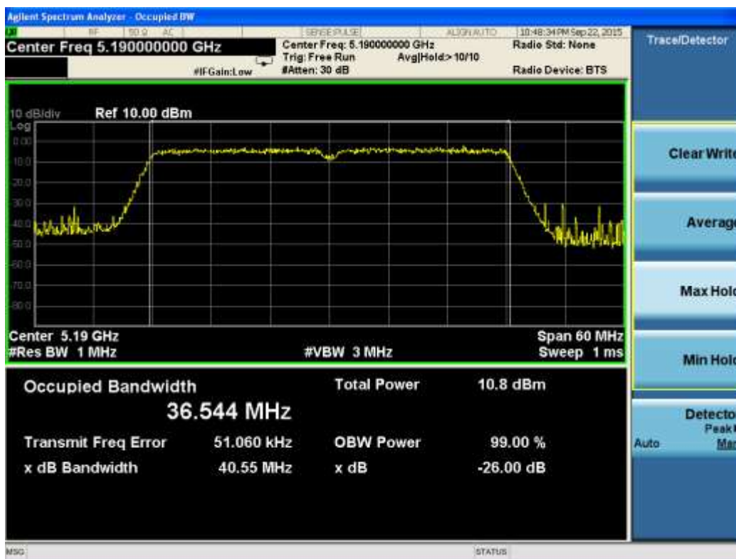
Test Plot For 802.11ac(VHT40)-26dB BW-5190M-Chain 0
