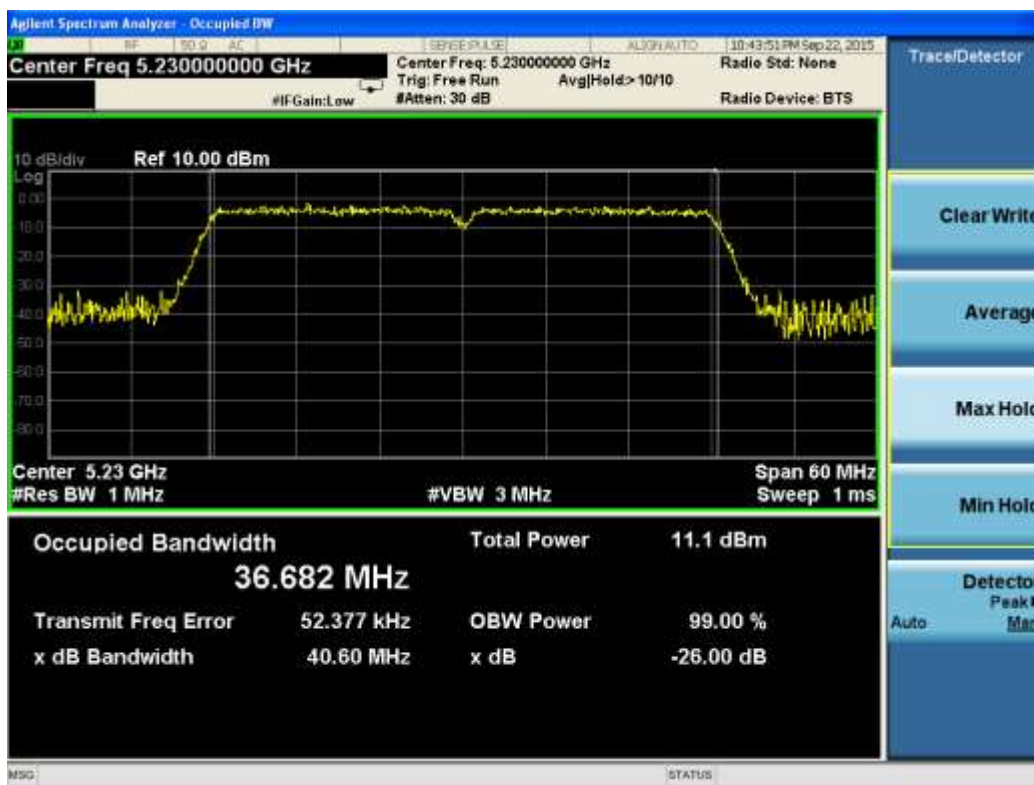
Test Plot For 802.11n(HT40)-26dB BW-5230M-Chain 0
