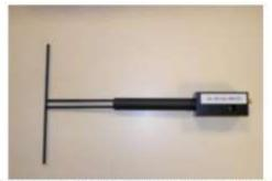
Figure 1 – Satimo COMOSAR Validation Dipole
