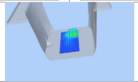
Test Mode:802.11A,MID channel(Body SAR-LCD DOWN)
