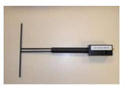
Figure 1 – Satimo COMOSAR Validation Dipole
