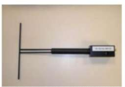
Figure 1 – Satimo COMOSAR Validation Dipole
