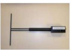
Figure 1 – Satimo COMOSAR Validation Dipole
