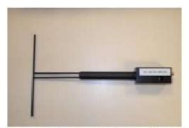
Figure 1 – Satimo COMOSAR Validation Dipole
