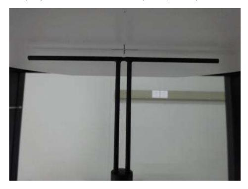
Photo of Dipole Setup
