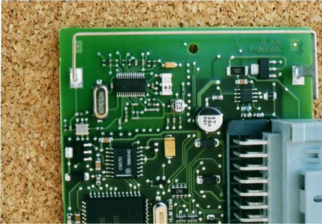
GQ43VT28R Receiver PCB RF Section Close-up Top
