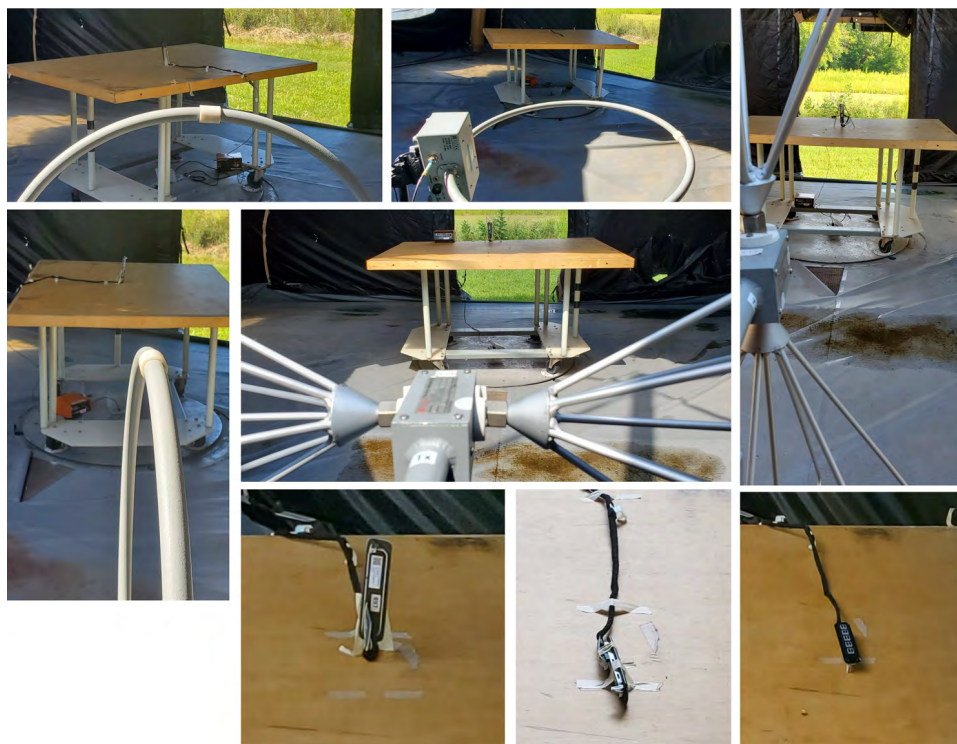
Figure 4: Radiated Emissions Test Setup Photograph(s).
