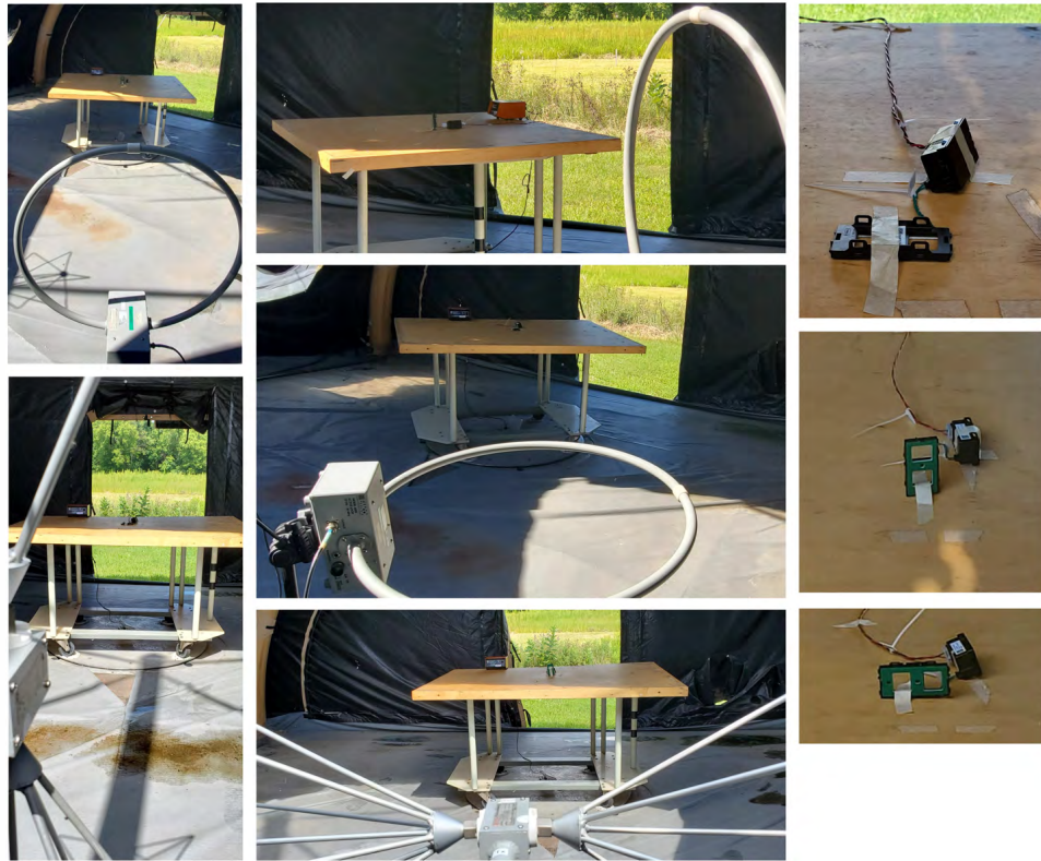
Figure 4: Radiated Emissions Test Setup Photograph(s).
