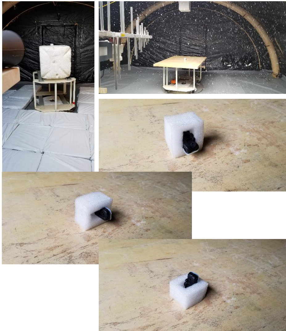
Figure 4: Radiated Emissions Test Setup Photograph(s).
