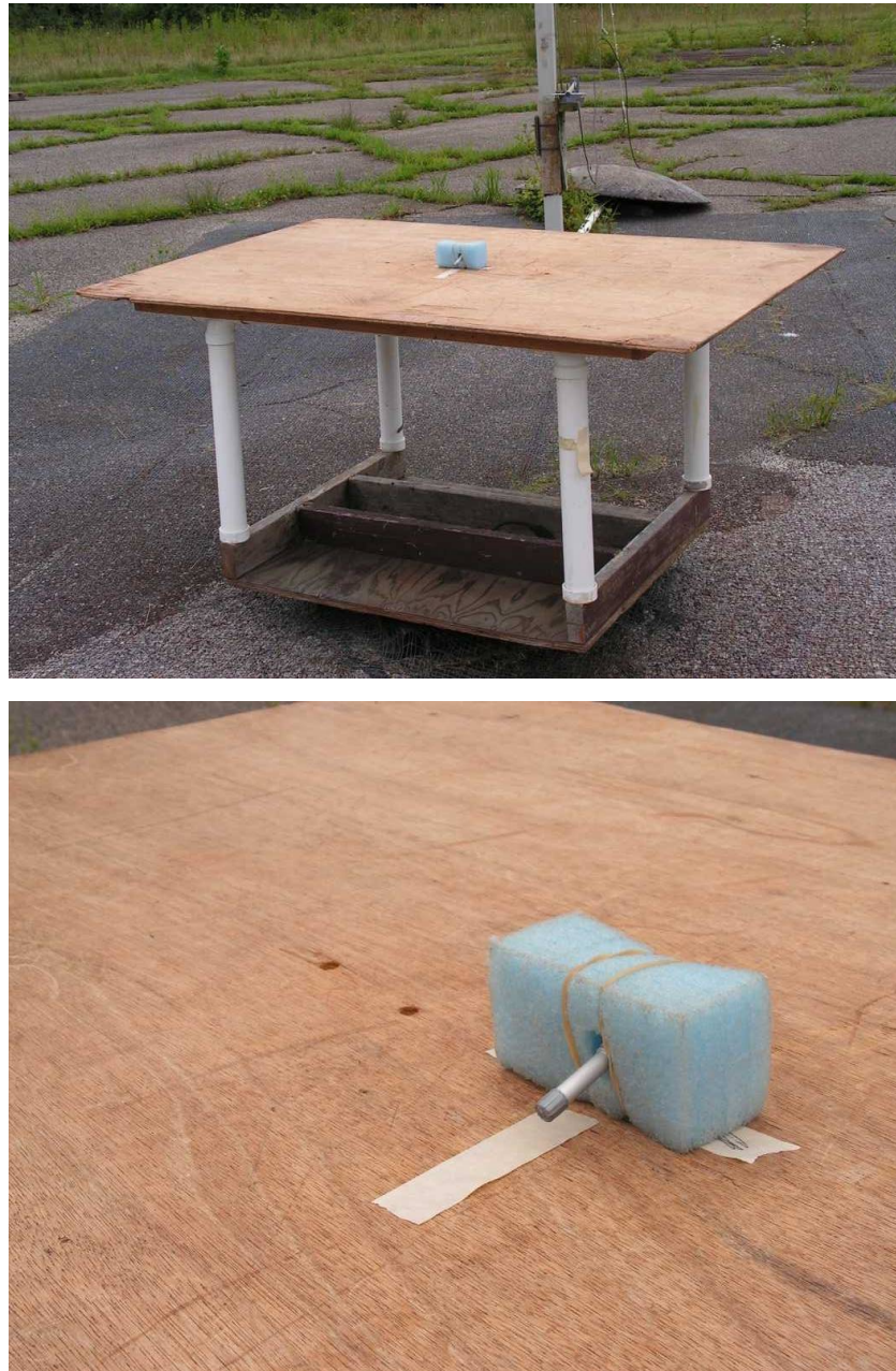
Figure 4: Radiated Emissions Test Setup Photograph(s).
