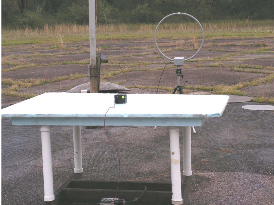
Photograph 6.4. DUT on OATS (one of three axes tested)
