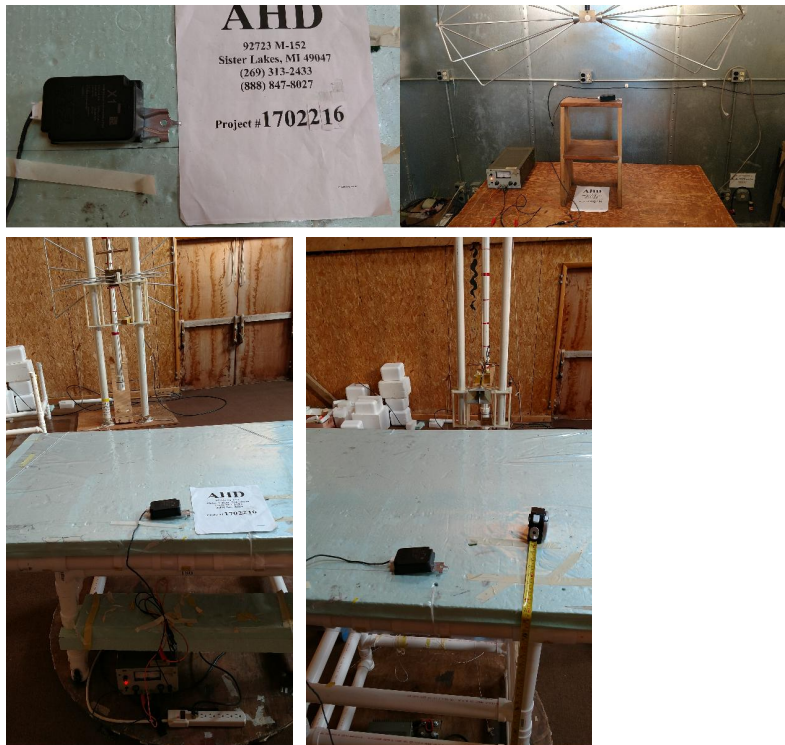
Figure 4: Radiated Emissions Test Setup Photograph(s).
