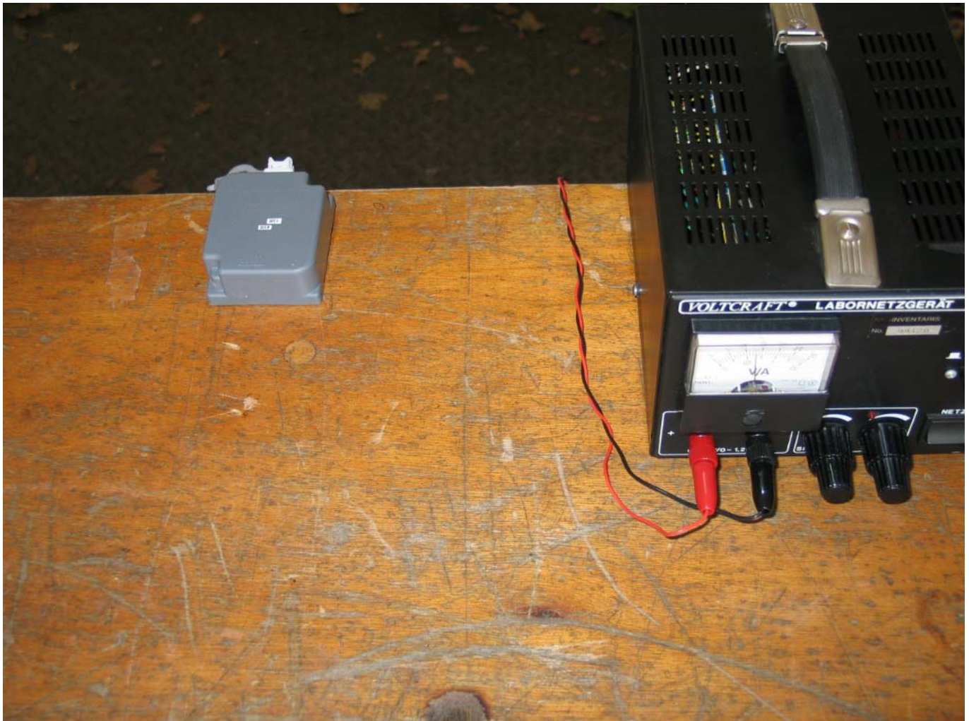
Photo 1: Radiated emission measurement set up
