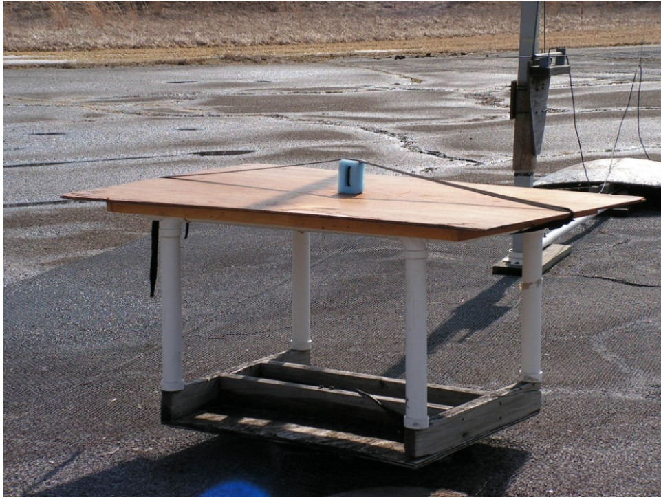
DUT on OATS – one of 3 axes tested
