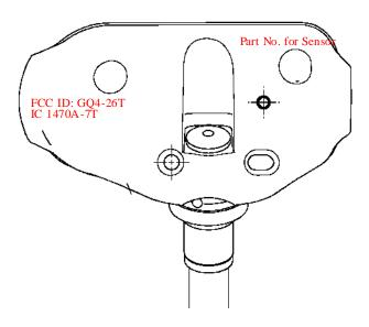
Figure 1. FCC/IC Identifier and Model Number
