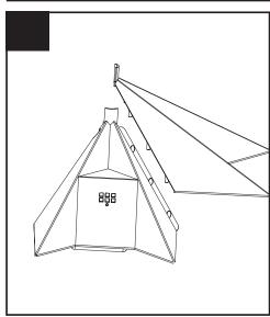
4. Attach base connector ring (  $\mathsf{E}$  ) over the top of the assembled base.
