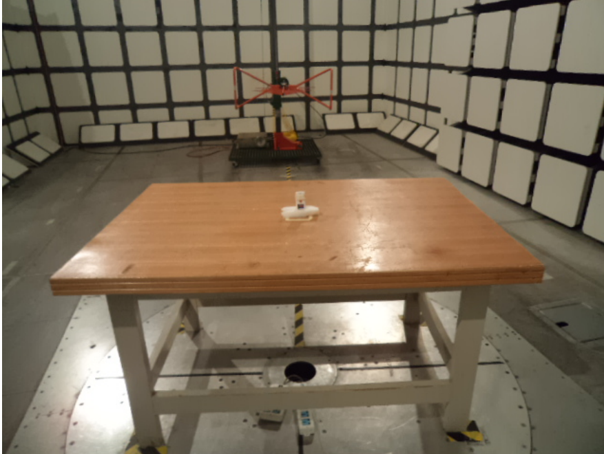
Radiated Emission View (Below 1 GHz)
