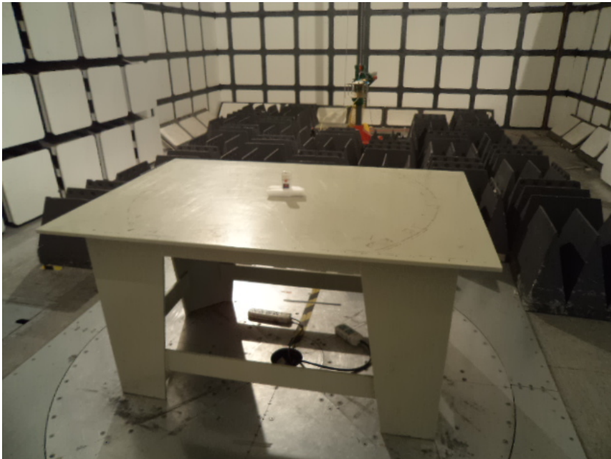
Radiated Emission View (Above 1 GHz)
