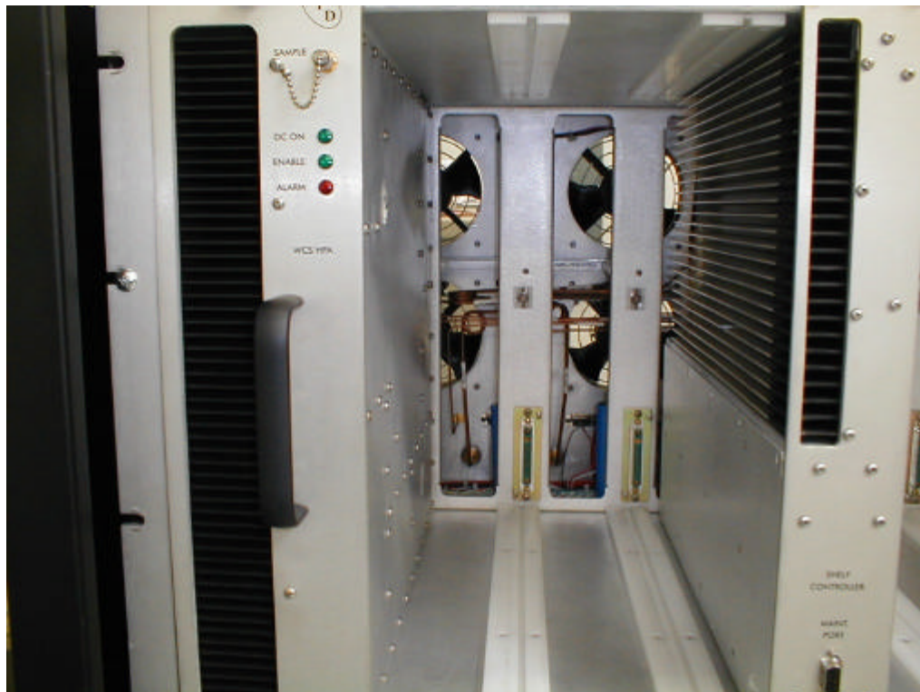
Power Amp Shelf; Left is PA #1, Right is PA controller.
