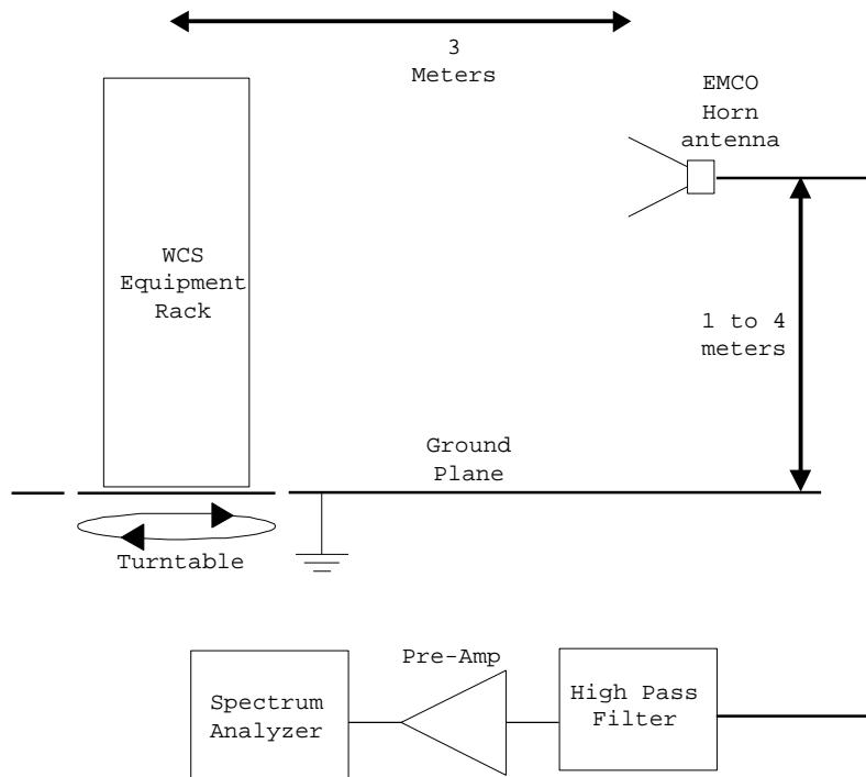
**Out of Band Emissions (Radiated) test setup.**
