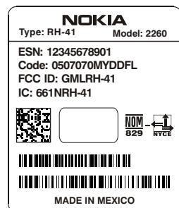
**NOTE:** ARTWORK PICTURES ARE ONLY EXAMPLES; IN PRODUCTION THE CORRECT DATA IS READ FROM THE TRANSCIEVER CAN BE PRINTED IN NMP PRODUCTION USING: FLEXCON TC-200V-156 MATERIAL & THERMAL TRANSFER RIBBON ZEBRA 5095 CODE 9730000.
