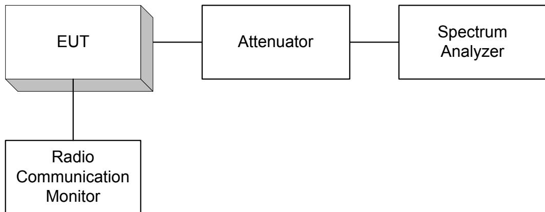
*The Radio Communication Monitor is used only to provide modulation input for external modulation.*
