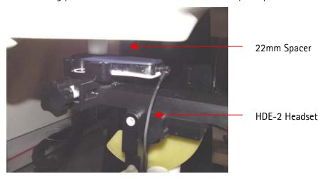
Note: the 22mm spacer was removed before the SAR measurement.
