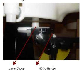
Note: the 22mm spacer was removed during the SAR measurement.
