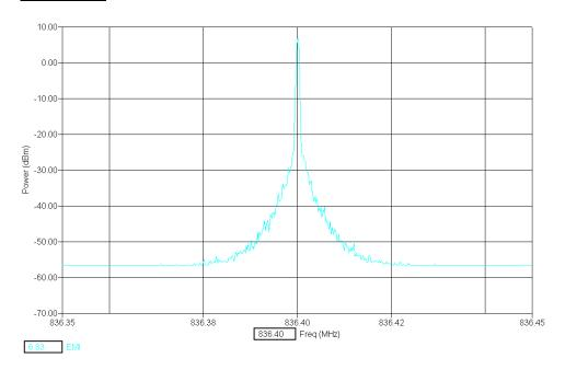
AMPS Min and Max Power – Voice (2500 Hz Sine Wave); F3E/F3D mask
