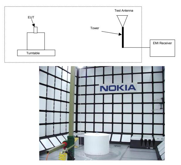
Test method is according to ANSI/TIA/EIA 603A.
