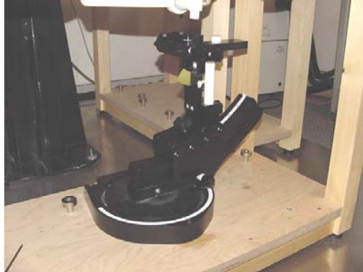
Device holder supplied by SPEAG
