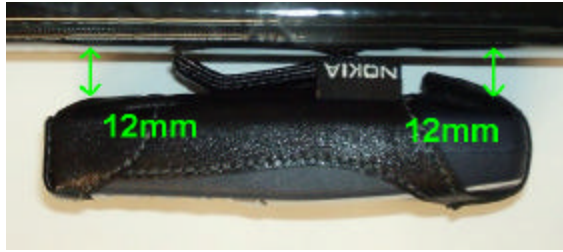
Picture 3. Separation distance with Leather Carry Sleeve CSL-12
