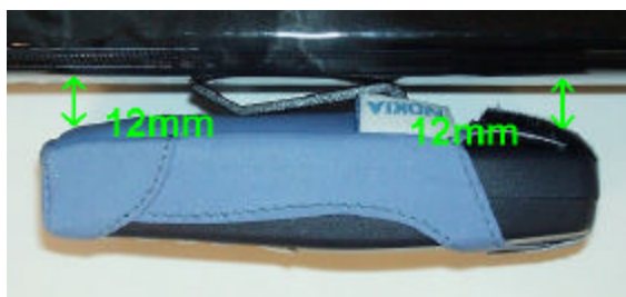
Picture 2. Separation distance with Carry Sleeve CSH-7
