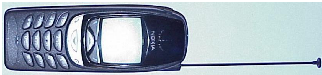
Figure 2 GMLNHP-2AX with antenna extended
