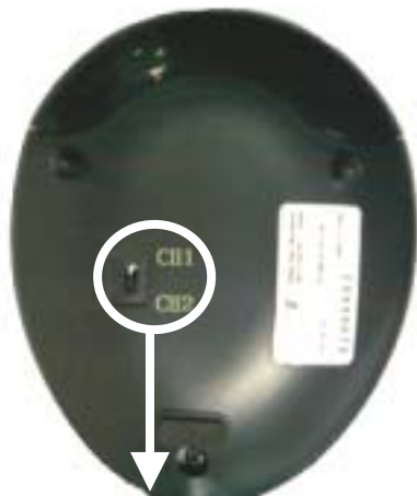
Receiver Channel Switch
