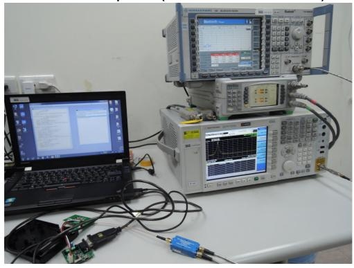
**Conducted Setup Photo (Measurement at Antenna Port)**
