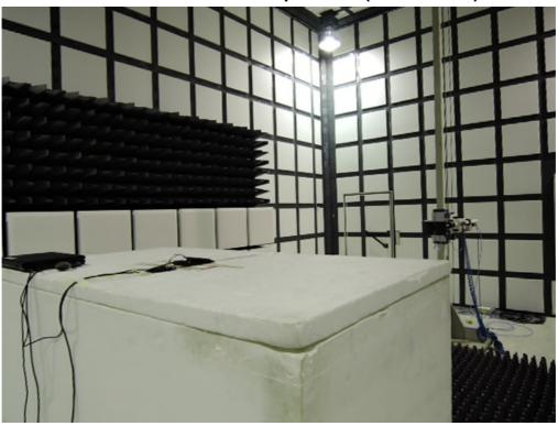
Radiated Emission Set up Photos (Above 1GHz)
