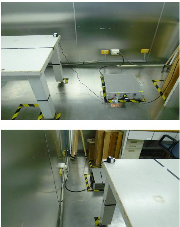
**AC Power-line Conducted Emission Set up Photo**
