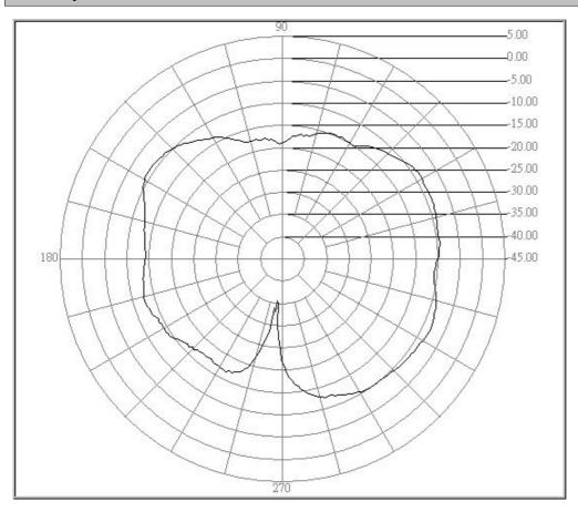
Center freq.(MHz): 2500 Polarization : E Plane
