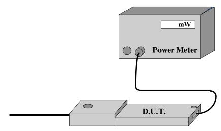
Measured Power  $\approx$  Measured Power + Cable and Switching Mechanism Loss
