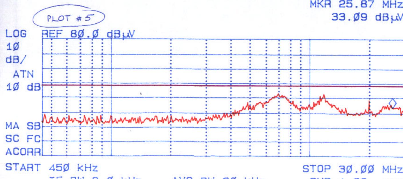
Test Configuration #5: Teklogix TRX7431 Radio installed inside Teklogix 9150 Base Station
