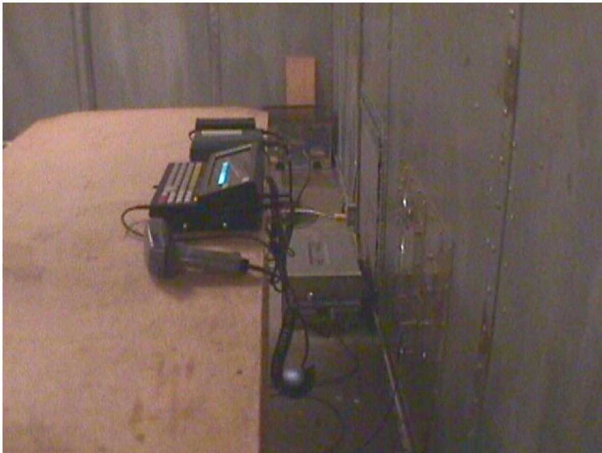
**Test Configuration #4 Setup: Teklogix TRX7431 Radio installed inside Teklogix 8260 Vehicle Mount**
