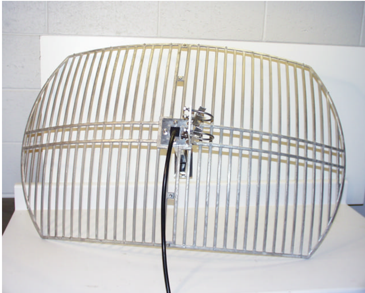
Photo #4: Conifer 26T-2400F Grid Disk, Gain 24 dBi
