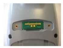
You can now install the RFID Module UHF-CAQ-AC5-NEO.
