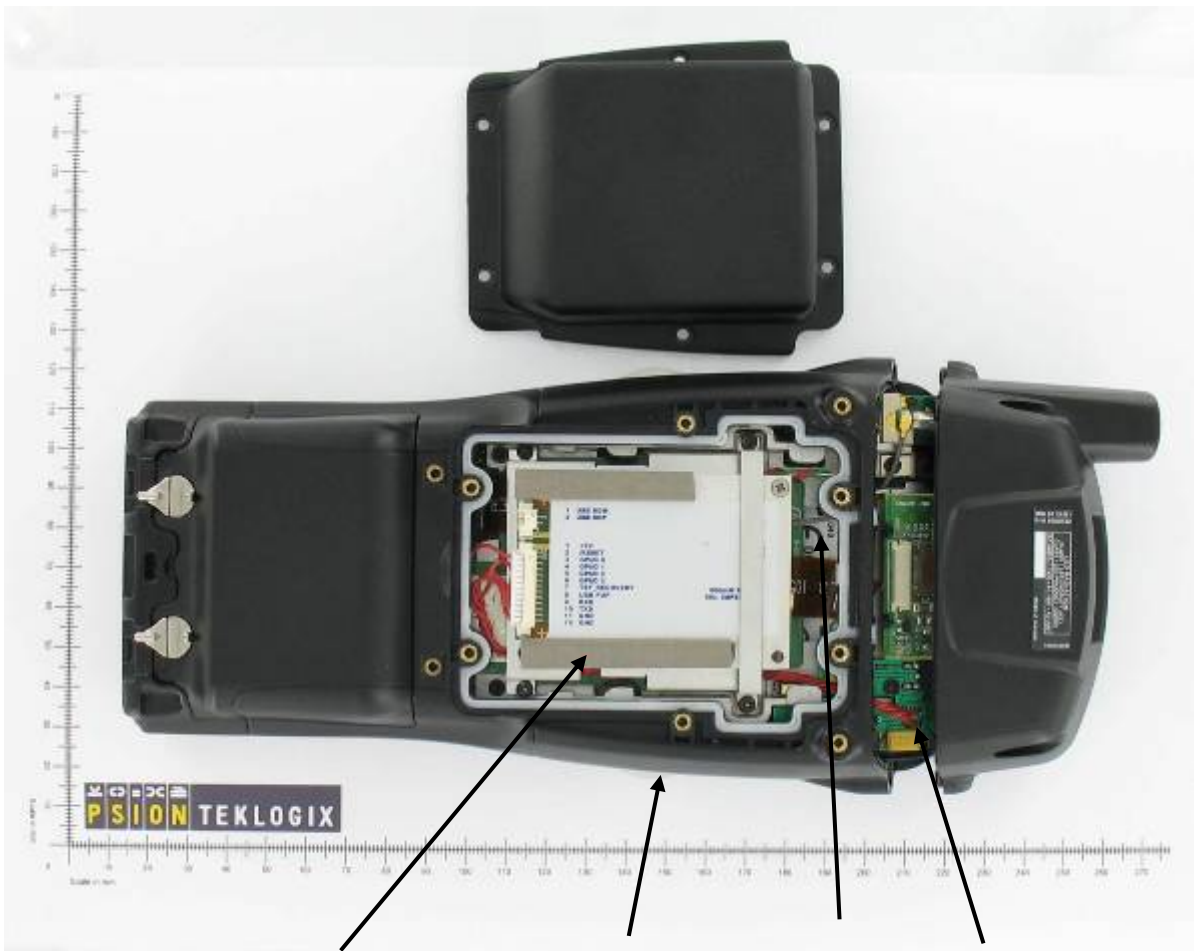
RFID Module Bluetooth on the Main logic board (native on the WAP) WIFI RA2041 on the CF-card slot interface board
