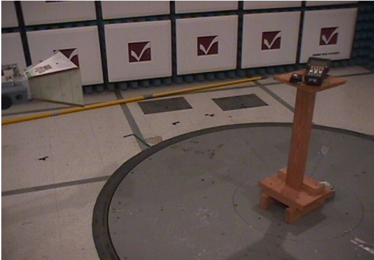
View of the Scanner during the Radiated Emissions tests. This view shows the sample during the 1 meter measurements above 5 GHz.
