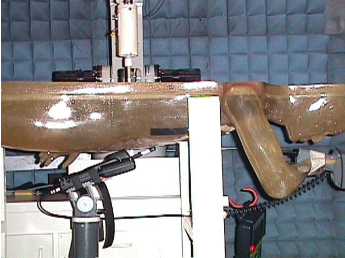
< Overview – Waist with the tip of the antenna in contact with the phantom and the display faced outward from the phantom >
