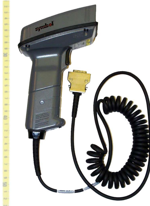
< Handheld laser scanner, M/N:LS-3200-I300A >
