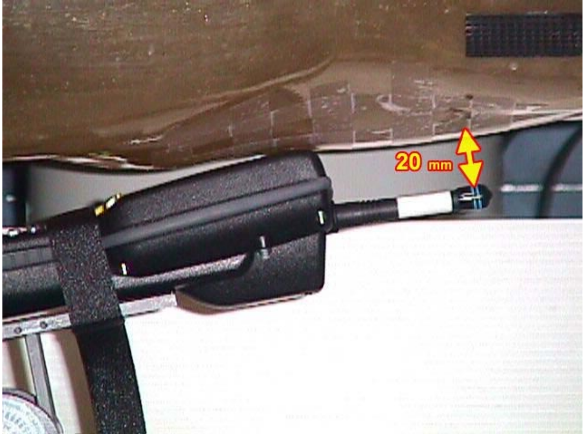
< Close-up view – Waist with the EUT parallel to the phantom and the display faced inward to the phantom >
