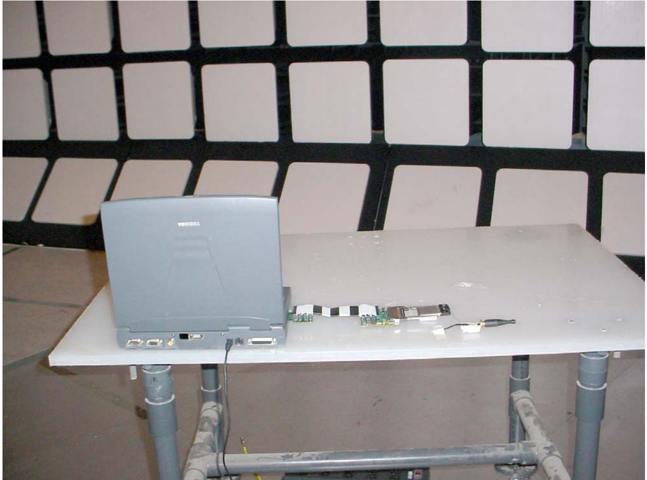
Radiated Emissions at 3 m (RA2040 with Straight Dipole Antenna)
