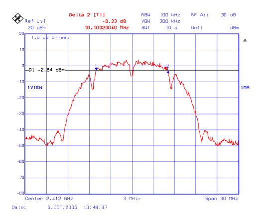
Plot 6.6.5.5 6 dB Bandwidth Frequency: 2437 MHz; Modulation: DQPSK; Data Rate: 2 Mbps
