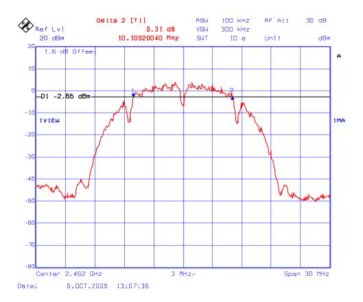
Plot 6.6.5.7 6 dB Bandwidth Frequency: 2412 MHz; Modulation: CCK; Data Rate: 11 Mbps
