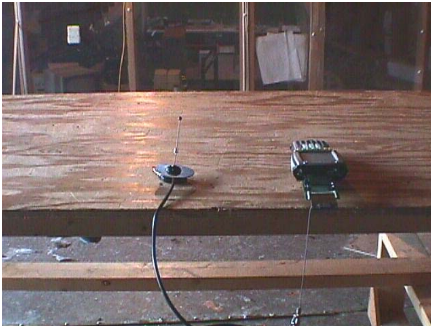
Test Configuration #2: Psion Teklogix Model RA2020 + Mobile Mark Antenna, Model IMAG5-2400, Gain: 5 dBi
