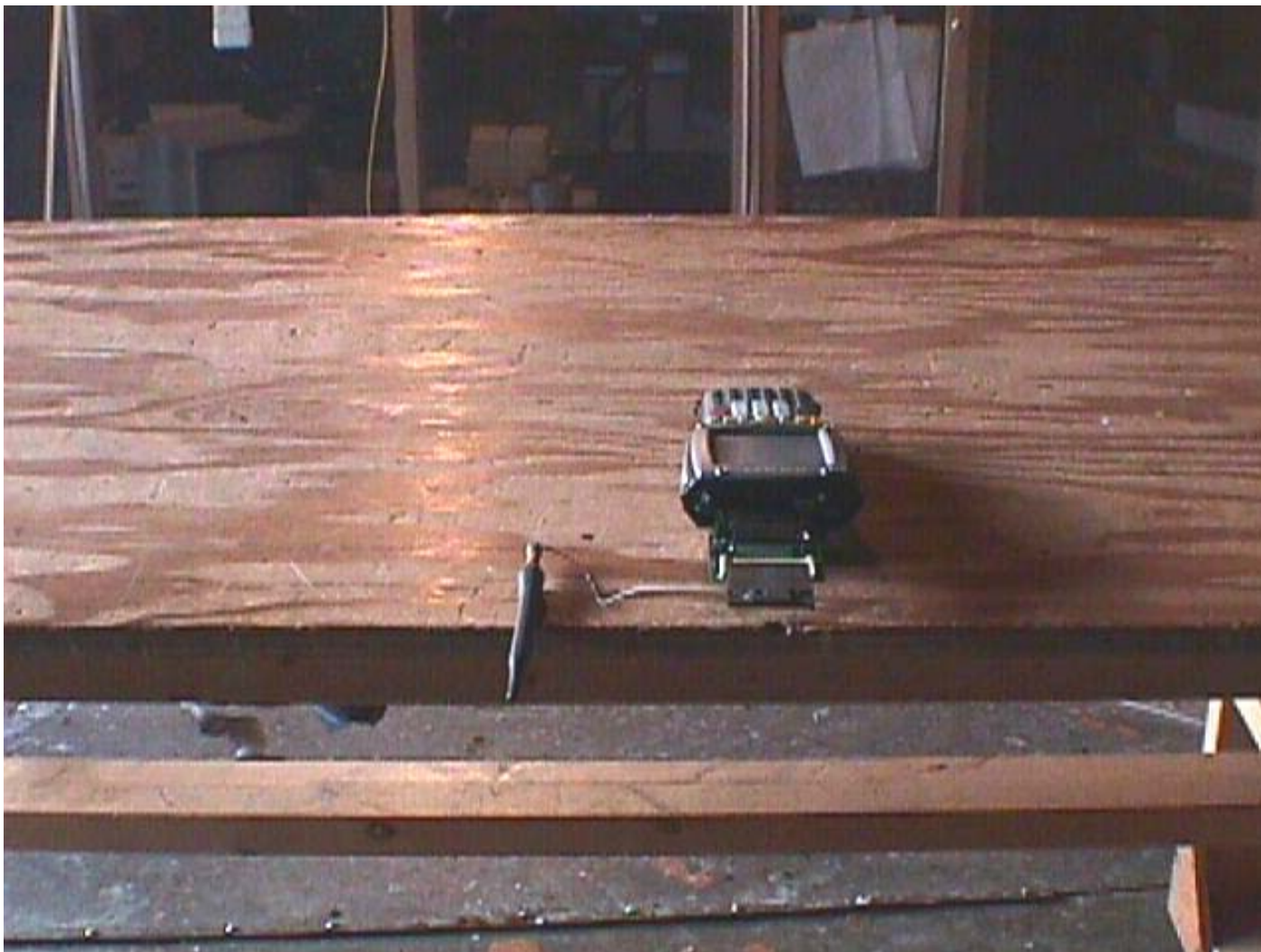
Test Configuration #1: Psion Teklogix Model RA2020 + Radiall/Larsen Antenna, Model EPA 02-016, Gain: 2 dBi
