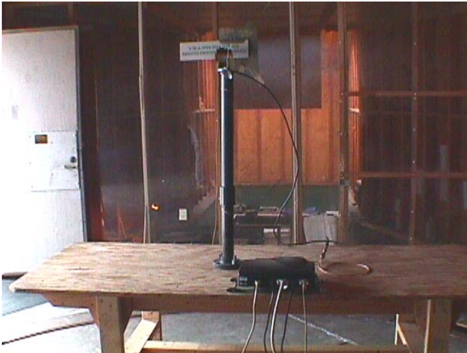
Test Configuration #2: Psion Teklogix Model No.: 9150-RA2020 + Mobile Mark Antenna, Model IMAG5-2400, Gain: 5 dBi
