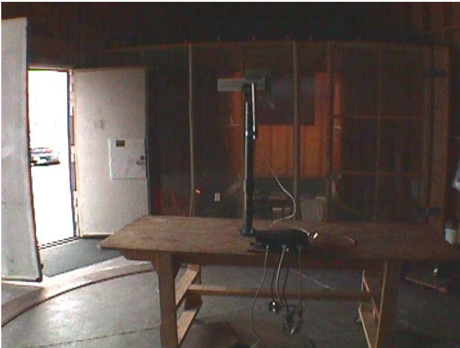
Test Configuration #3: Psion Teklogix Model No.: 9150-RA2020 + Cushcraft Antenna, Model S24003BP12NF, Gain: 5.2 dBi
