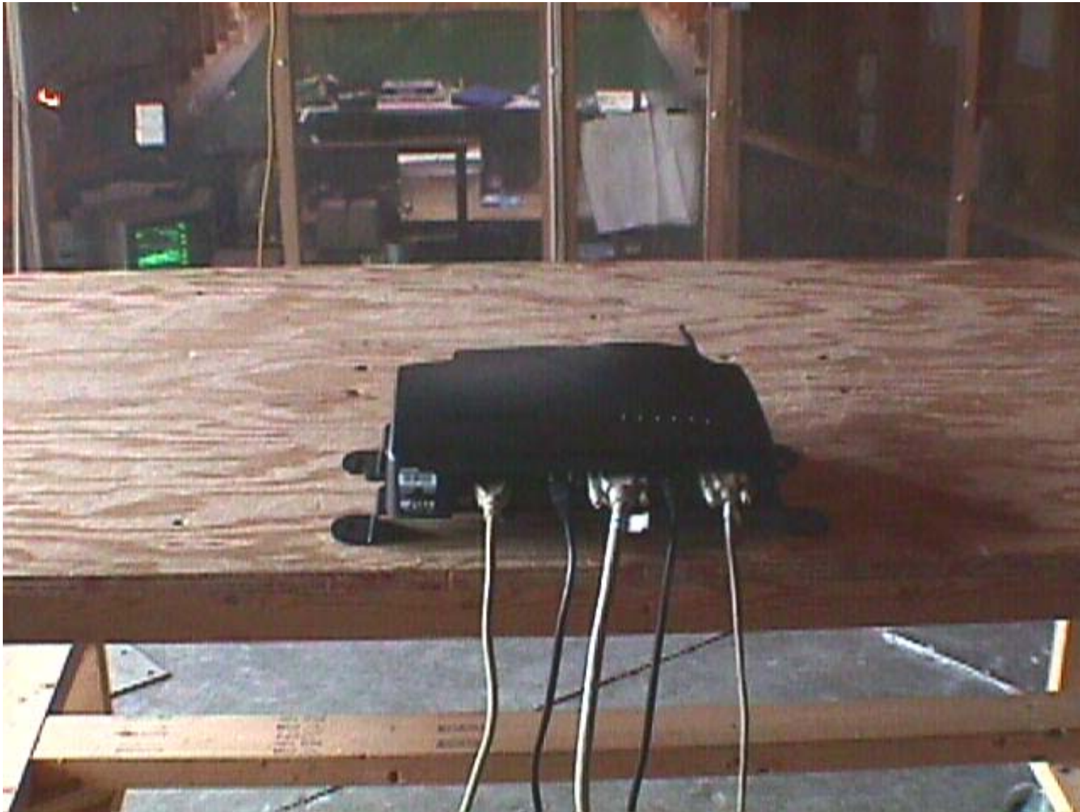
Test Configuration #1: Psion Teklogix Model No.: 9150-RA2020 + Centurion Antenna, Model EXE-2400-SMRP, Gain: 2 dBi
