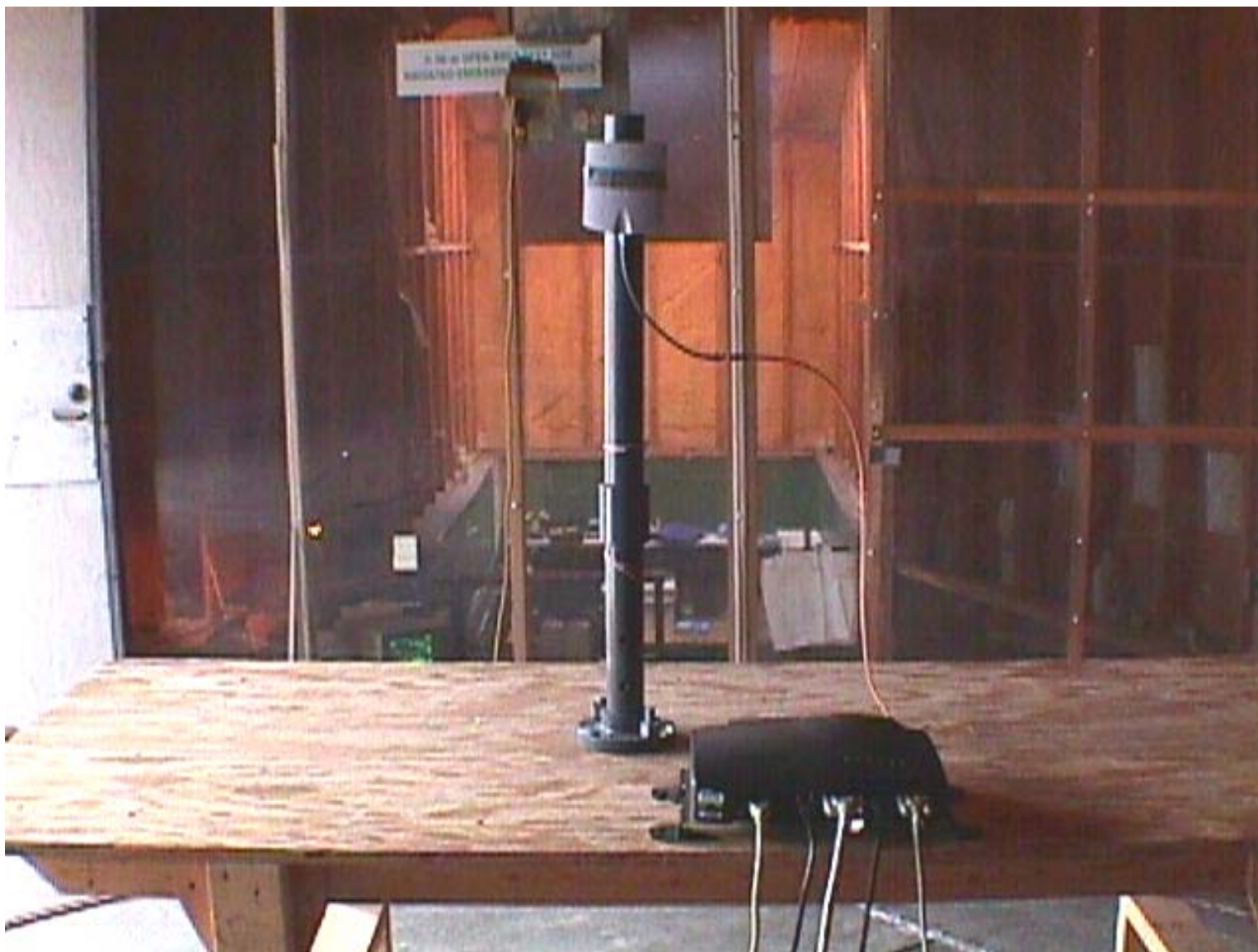
Test Configuration #5: Psion Teklogix Model No.: 9150-RA2020 + Cushcraft, Model S2307AMP10SMF, Gain: 7.5 dBi
