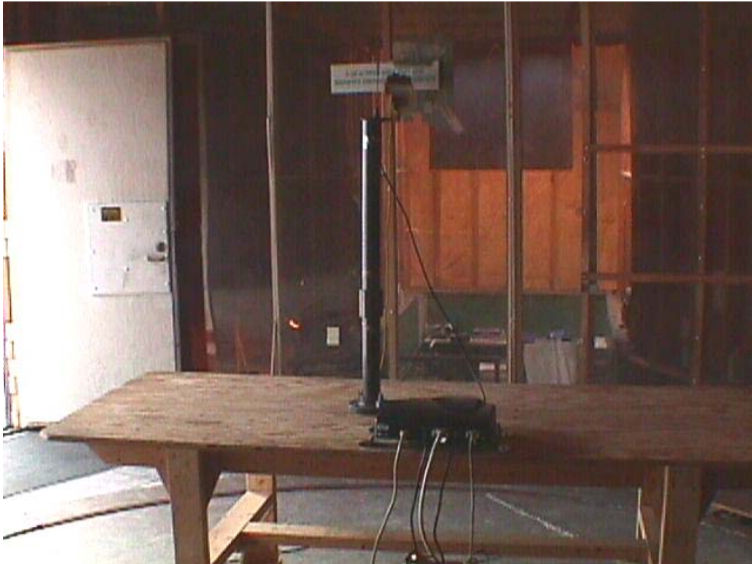
Test Configuration #4: Psion Teklogix Model No.: 9150-RA2020 + Larsen Antenna, Model FB45T2400, Gain: 7.2 dBi
