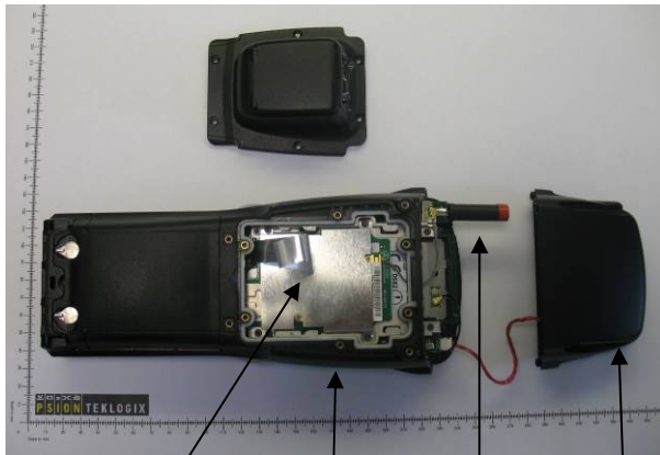
GPRS RA3030-G2 BlueTooth On the Main Logic Board (Native in the WAP G2) GPRS Antenna RFID Module
